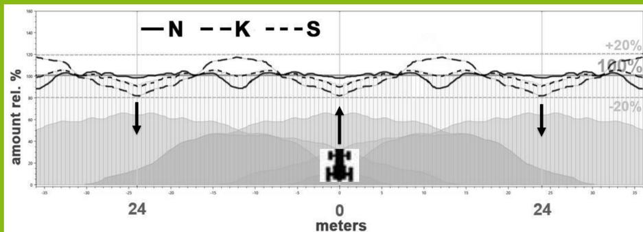
24m-spreading pattern (720 rpm, drop point 20): rate, nitrogen (N), potassium (K) and sulfur (S)
