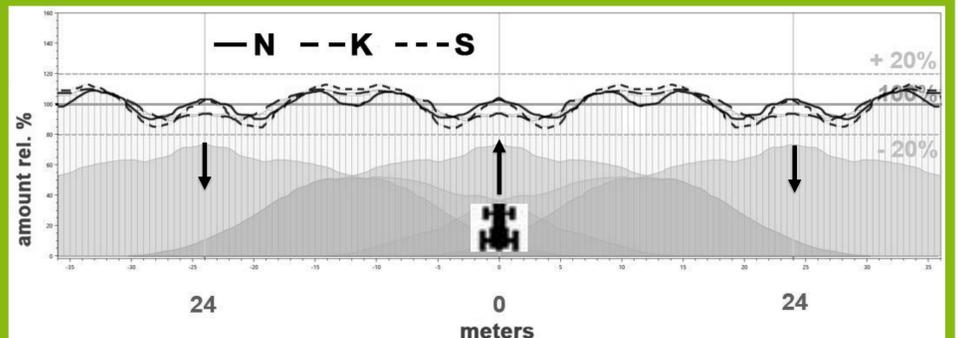
24m-spreading pattern (720 rpm, drop point 20): rate, nitrogen (N), potassium (K) and sulfur (S)
